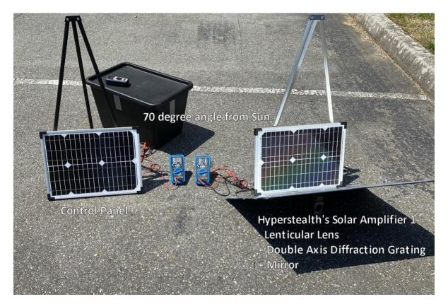
The #2 Amplifier with the double axis diffraction grating removed so it is a lenticular lens over a mirror as seen in the second photo in this article, still functions nearly equal to the one with the addition of the diffraction grating when pointed directly at the sun, but drops off substantially when angled away.
