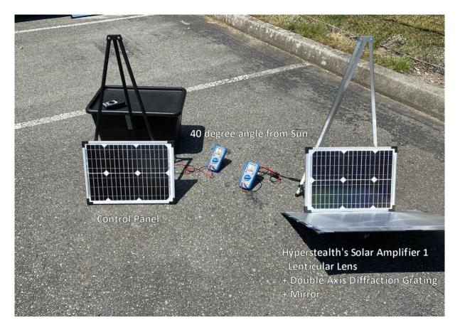
And changing the horizontal (left/right) angle to 70 degrees to simulate even later in the day demonstrated a boost of 123.36% (more than double) from the amplified panel over the control panel at the same angles. When compared to the initial control panel facing the sun, the boosted panel at these angles provided 35.02% less power, while to control panel at these angles lost 71% of the power output compared to the control panel that faced the sun.
