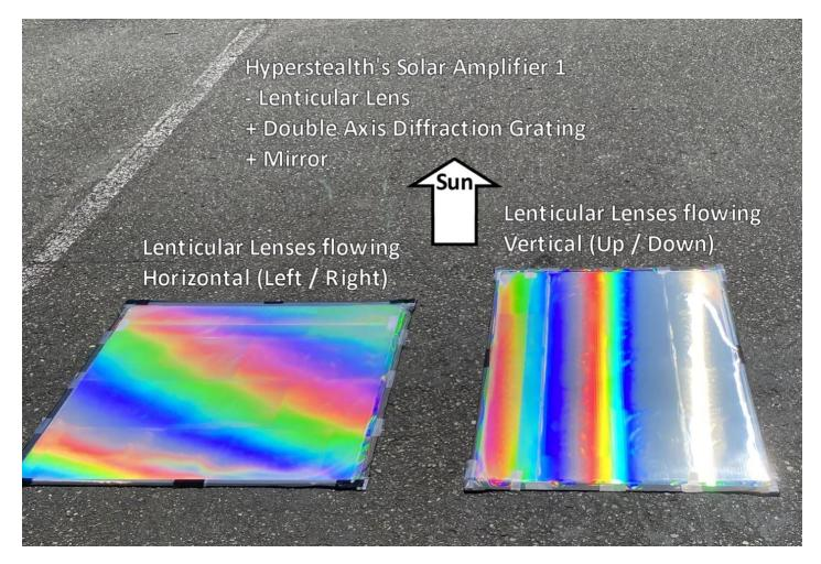
This passive amplifier consisted of a mirror with a double axis diffraction grating layer and a lenticular lens. The double axis diffraction grating combined with the lenticular lens is what causes the light to bloom because it splits the light into different parts of the color spectrum causing the rainbow or prism effect, the mirror then reflects back any light that gets through the layers.
